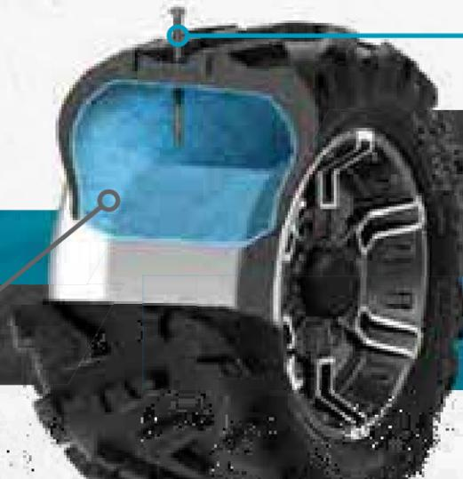
Once a leak occurs, the tire sealant rushes out of the tire and quickly creates a permanent solid plug.
