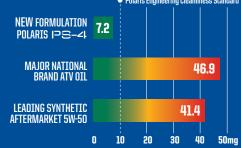
ASTM D6335. In 3rd party against 9 competitive products Polaris PS-4 had less than half the deposits compared to the next closest product. No other tested products met Polaris Engineering standards for deposit cleanliness.
