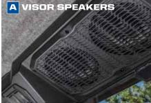
Four 16.5 cm speakers located in the overhead Waterproof system for reliable power and sound quality
