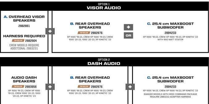
AUDIO DASH SPEAKERS INCLUDE BUILT-IN FOUR CHANNEL AMPLIFIER (40-WATTS) AND TWO OFF-ROAD GRADE 13.3 cm SPEAKERS
